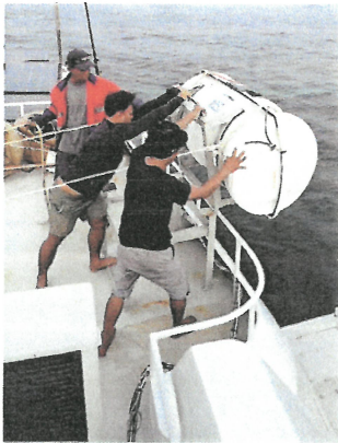
Here, the crew is seen removing the life raft pod for sending it to Benoa Port for servicing.
