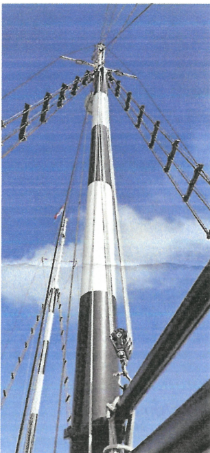
Looking closely at this photo, one can see both the cable shrouds and the sheet lines that we will be renewing in March.
